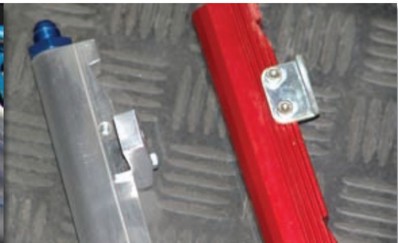
A pair of LS1 fuel rails. One has the correct mounting brackets to stop flex, and one doesn't. Can you pick which one is which?
