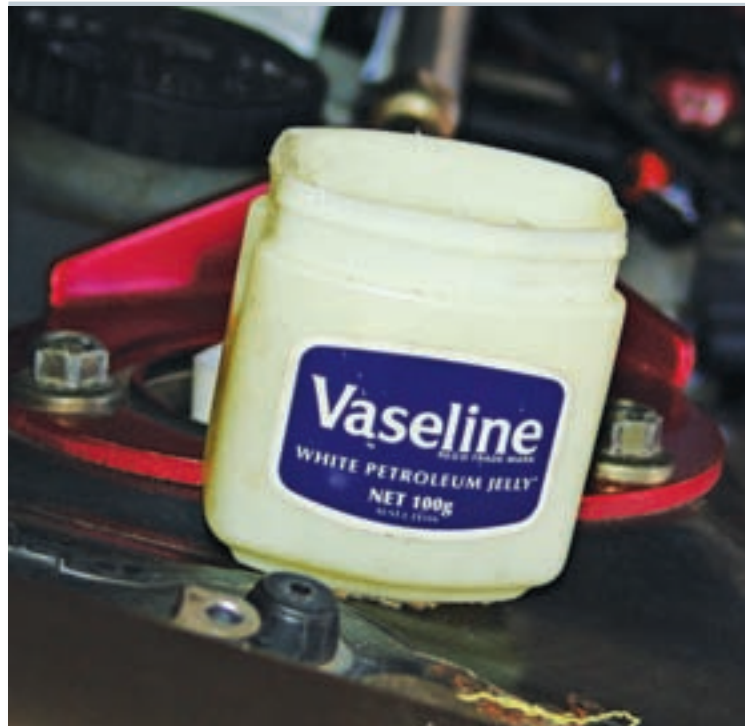
A touching process – applying good old vaseline to the injector O-rings to stop them grabbing
