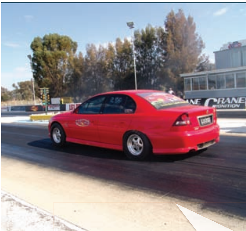
Notice the Ute's turbocharged cousin, which makes twice the power (and then some) of the bolt-on car. It has much less of a squat off the line and simply drives away to a 10.5sec pass
