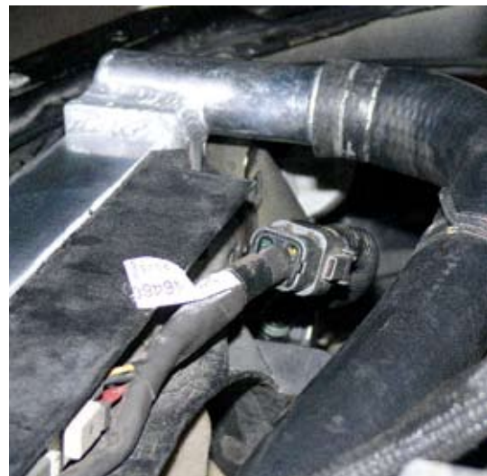
6 With the radiator in the car, the hoses are then connected and the mounting clips are put back on as per the factory radiator. We left the top radiator hose off so that we could bleed the system properly, then put it back on and continued to fill it with water
