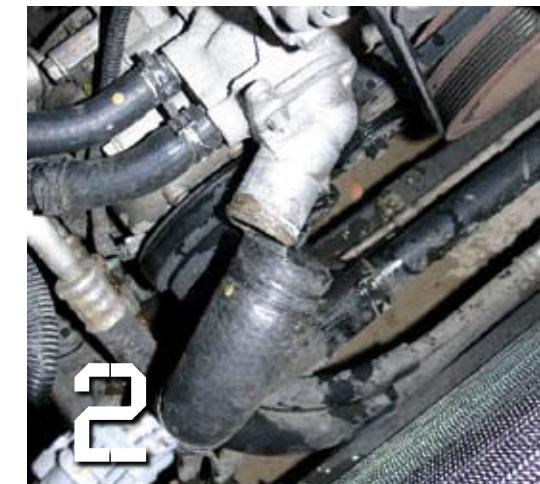
2 With the car having sat for a while, there was no excess pressure in the cooling system, so the radiator hoses could be undone and the water drained out of the system. In a typical automatic car, the transmission cooler lines will also need undoing and propping up so that trans fluid does not drain everywhere
