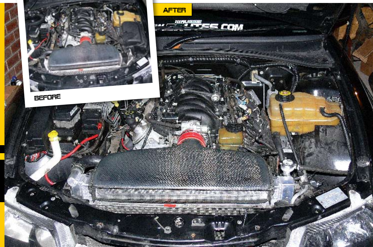
6 With the radiator in the car, the hoses are then connected and the mounting clips are put back on as per the factory radiator. We left the top radiator hose off so that we could bleed the system properly, then put it back on and continued to fill it with water
