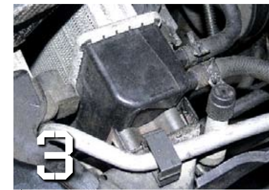
3 There is a pair of metal clips (one on either side of the radiator), which can be removed with a flat-head screwdriver, and with the thermo fans unplugged or unscrewed from the radiator, it should slide straight out the top
