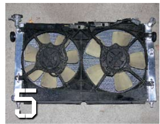
5 With the new JAR radiator sitting on the ground, you can see that all the mounting tabs and screws line up perfectly. The fans are secured to the radiator as per factory so that it can then be slid back into the car
