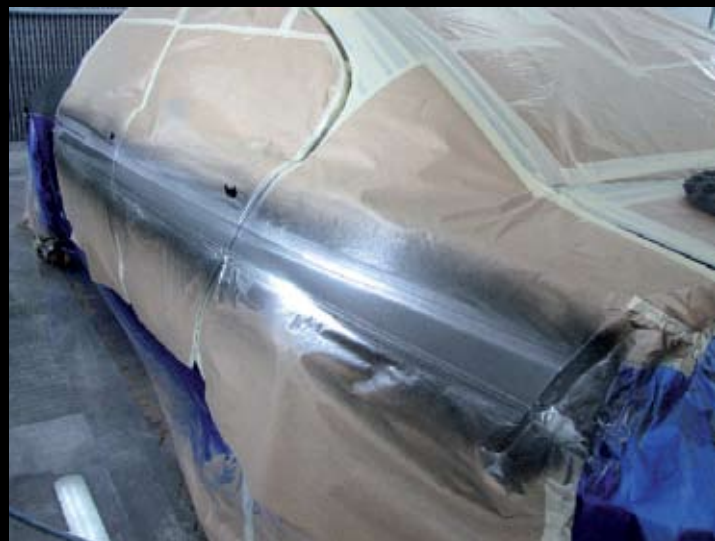
This is what the car looks like before the Flo-Clear clear coat is applied. Even at this stage, it's apparent how vibrant the colours are. Notice that the factory-black top half is getting cleared as well
