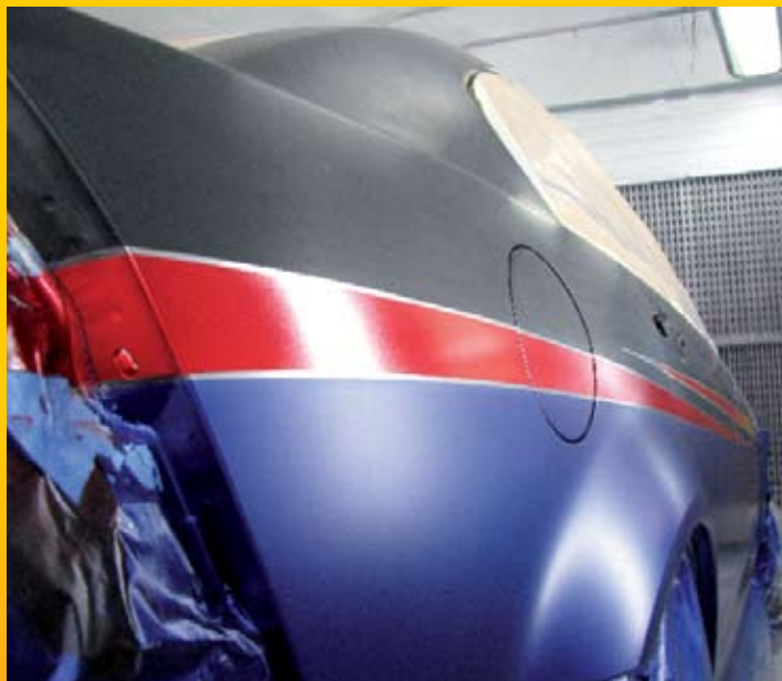
This is what the car looks like before the Flo-Clear clear coat is applied. Even at this stage, it's apparent how vibrant the colours are. Notice that the factory-black top half is getting cleared as well
