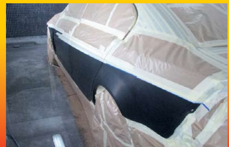
With the design marked out, the top half of the car (or whatever half is not receiving paint) is masked off
