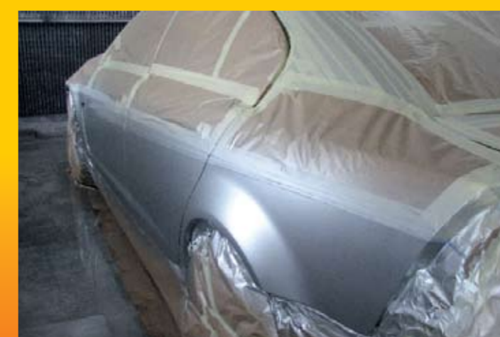
The first colour to go on the car is Orion Silver that will form the base colour for all three candy paints. As Owen explains, a vibrant base colour like the Orion silver will make the hue laid over the top appear clearer and more vibrant
