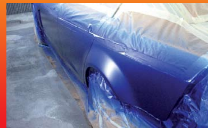
Over the top of the silver goes the Cobalt Blue Kandy, which is making up most of the car's lower half
