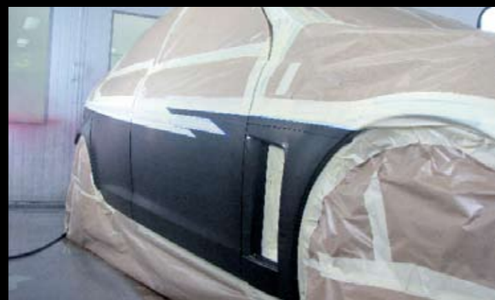
Masking off is an intricate process and very time consuming, but if a two-tone job is going to work, you need to make sure you get it right. There's never an 'it'll do' or a corner cut, and that attitude gets the best results
